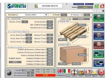
"Smart-Setup" management software that allows, by setting box and pallet size, the creation of the palletizing scheme/recipe independently in a few minutes.
